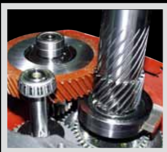
5HP heavy cutting milling head transmitted by gears
