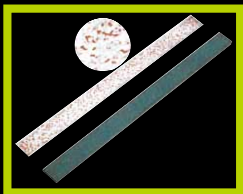
Strict hand scraping (16 point per square inch) Turcite-B coated on X & Y gibs
