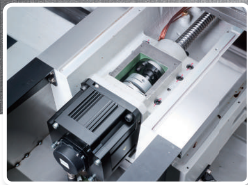
■ Axes motors are direct coupled with ballscrews, featuring high efficient motion control, high response and low noise.
