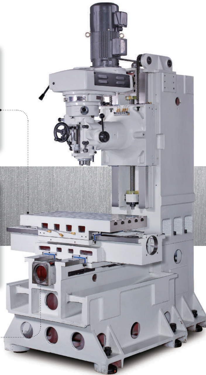
■ Axes motors are direct coupled with ballscrews, featuring high efficient motion control, high response and low noise.
