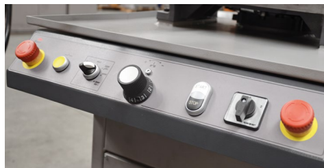
The central panel includes all of the control elements; it is located at an ergonomic height directly at the front of the machine
