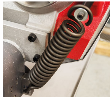
Flexible spring for easy movement of the arm to the cut and returning back to the top position
