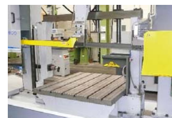
T-grooved clamping plate for free tensioning.
