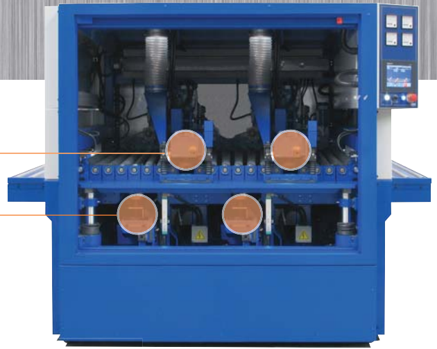
MB4 machine with 4 working units (two top & two bottom units)
