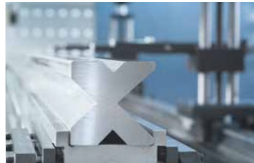
European Type Tool and Holder (4V Bottom Tool) Quick Clamping
