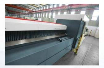
For longer parts than 800 mm, unloading table enters the cabin and unloads the parts.
