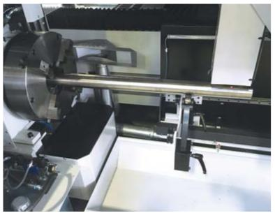
Pipe and tube profile rotation system Pipe diameter capacity of Ø30 up to Ø400 Square profile capacity of 250x250 Fume extraction connection Adjustable support units for pipe and tube profile
