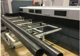
Tubes up to 6 m of lenght are removed by automatic unloading system with conveyor.
