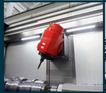
**Milling spindle.** For stable, precise and flexible drilling and milling operations. Up to 80 kW and 630 Nm of torque and 10000 rpm. Sealing air, internal HP coolant with 40 bar and externally with 14 bar and a 1400 liter paper band filter system as standard (80 bar option). The B-axis can be used at any angle or with an indexed B-axis in 2.5° steps.
