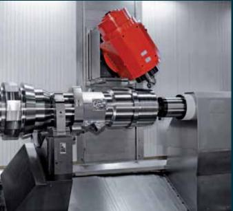
**Tailstock.** The tailstock is 100% programmable using the control. With the high-quality and precisely-dimensioned MK6 quill, all operations can be supported or extended with the counter spindle thanks to the machine modular construction.
