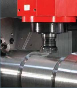
**Milling spindle.** Ready for use in the standard version with 6500 rpm for all turning, drilling and milling operations and technologies. The water-cooled ISM (integrated spindle motor) is available up to 80 kW and 630 Nm torque and with the HSK-T 100 or PSC80 (Capto C8).
