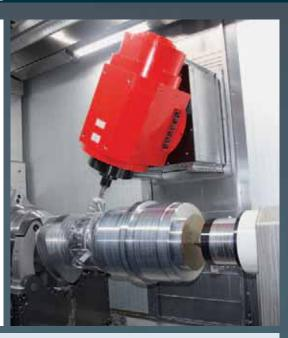
Milling spindle. Optional version with 10000 rpm. High speed for turning, drilling and milling operations, complex technologies usable for light alloys, aluminum, etc. The water-cooled ISM (integrated spindle motor) is available up to 80 kW and 340 Nm torque and with the HSK-T 100 or PSC80 (Capto C8).
