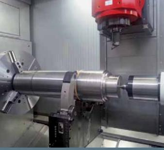
**Main spindle.** With performance data that make all machining possible without compromise. The EMCO spindle design has two servo motors that also act as C-axis. The motors operate in opposition, guaranteeing the balancing of the play and enabling the achievement of the power and torque as can be seen in the diagram above. The main spindle is also equipped with a special EMCO cooling system that optimizes the temperature stability and guarantees maximum precision with any length of machining.
