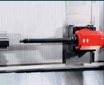
**Turning operations.** External or internal turning operations are possible with the stable spindle in 3° step. Optionally, the vibration-damped boring bar can be equipped up to a length of 1000 mm and with a 3-positions (stations) pick-up magazine.
