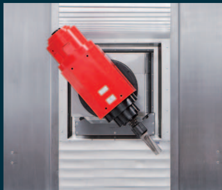
B-axis: The B-axis is driven by a torque motor, therefore achieving highly dynamic axis travel within the pivoting range of +/- 120 degrees.
