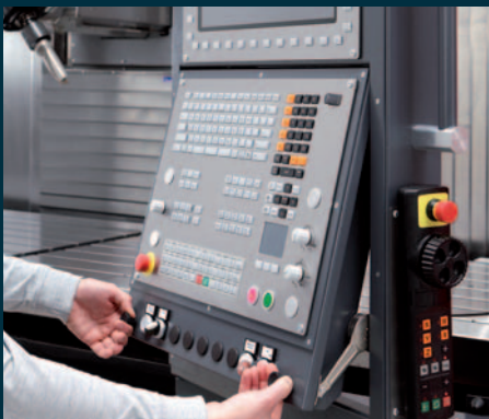
Control unit: The operator panel can travel, rotate and be adjusted in the direction of the work space. This ergonomic design provides ideal working conditions for the operator.
