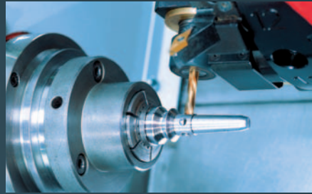
With 12 stationary and up to 6 driven tools, the EMCOTURN E25 offers an astonishing cutting performance – with top precision.
