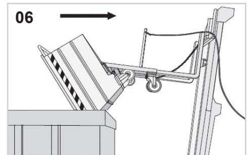
06 Move back in order to overlay the skip tilting container to the edge of the container
