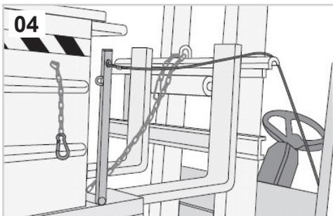
04 Place the release lever rope near the driver's seat
