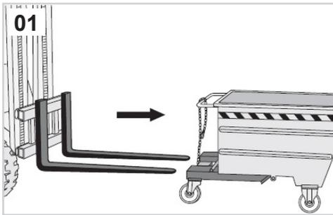
01 Place the forks into the appropriate fork jackets positioned on the bottom of the skip tilting container
