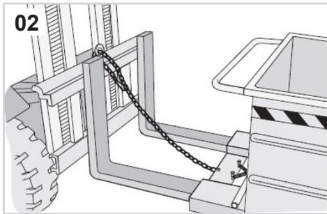
02 Connect the safety chain of the skip tilting container to the front crossbar of the fork carrier
