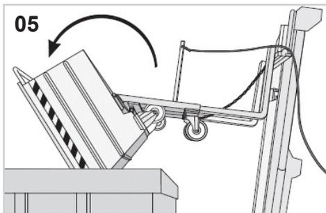
05 To unload the container: lift the skip tilting container just over the scraps collection container. Move forward with the fork lift truck until the skip tilting container is overlayed to the collection container. To unload the scraps pull the rope in order to operate the release lever of the container
