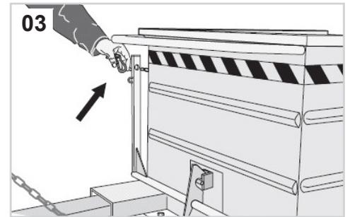
03 Remove the safety carabiner from the release lever of the container
