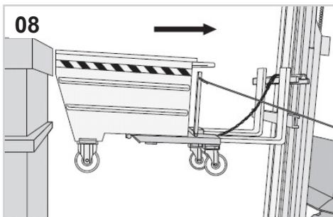
08 The container automatically returns to an horizontal position hooking up again the mechanical stop. Reposition the safety carabiner to the release lever.
