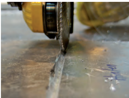
Milling a root gap by using the weld root opener
