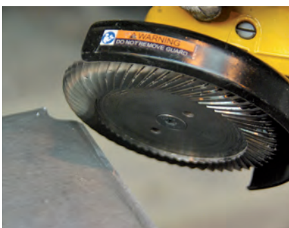
Making a bevel with a milling ring
