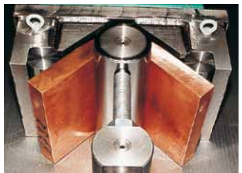
78 Dicke Platten biegen CU 300x40 R=40mm Bending huge flat material
