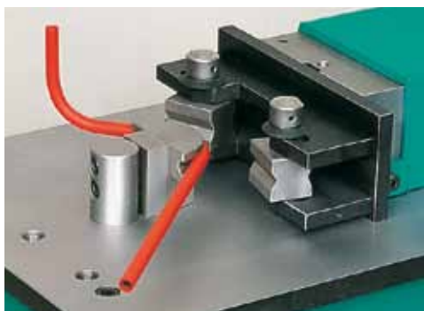
75 Hydraulikrohr biegen Hydraulic pipe bending
