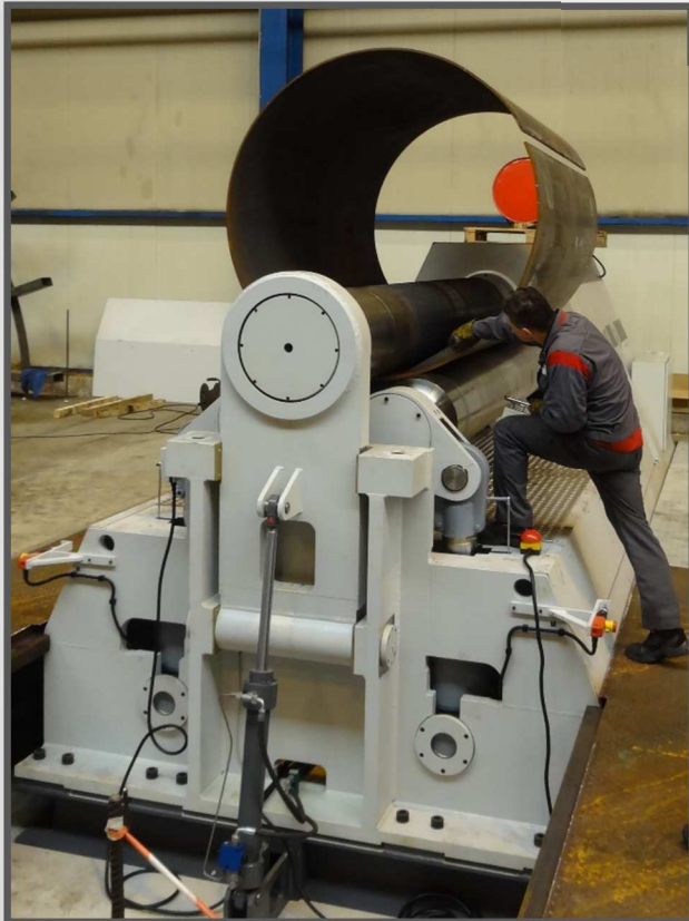
PB3-18-10 (top roll Ø457 mm, length 3050 mm)
