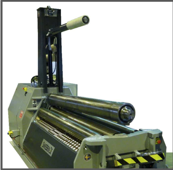
PB4-8-6 with hydraulic lifting roll in highest position
