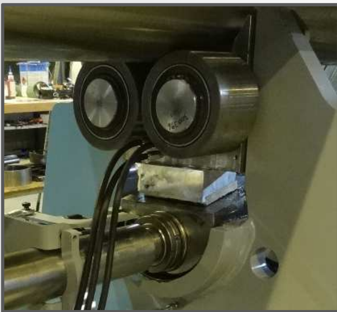
Powered support rolls (optional equipment) under the lower roll to "adjust" roll crowning and compensate for roll deflection.
