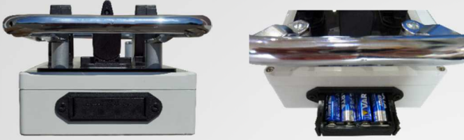
Wireless control unit uses four standard AA (LR6) batteries
