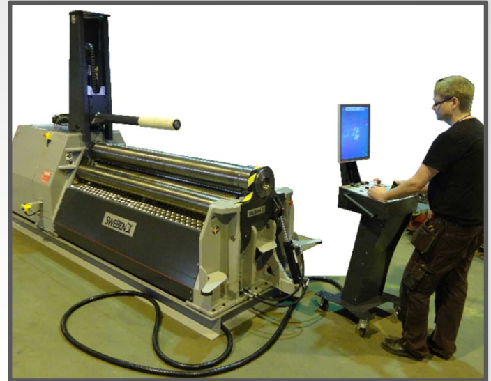
PB4-8-6 (top roll Ø203 mm, length 2000 mm) Equipped with CNC, hydraulic lifting roll & powered support rolls under the lower roll
