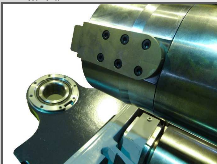
Cone bending device with hardened key Hardened cone roller is also available if desired
