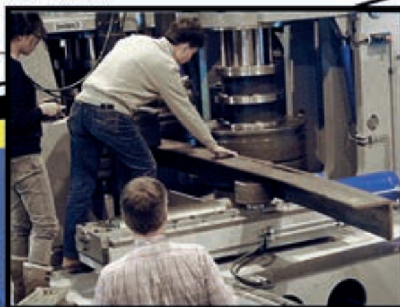
L200x200x20 in the Vertical Section Bending machine VSB3-400-3200
