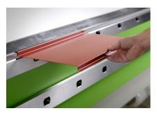
Master of fine detail. With the CIDAN concept of spring steel gauging fingers and the narrowest folding rail on the market, you get precision, finish and flexibility, even for very fine gauge measurements, down to 3 mm.
