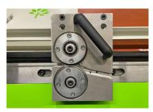
With a simple **rotary shear** attachment along the bend line, you can easily cut off blanks or folded profiles. (Only F41.)
